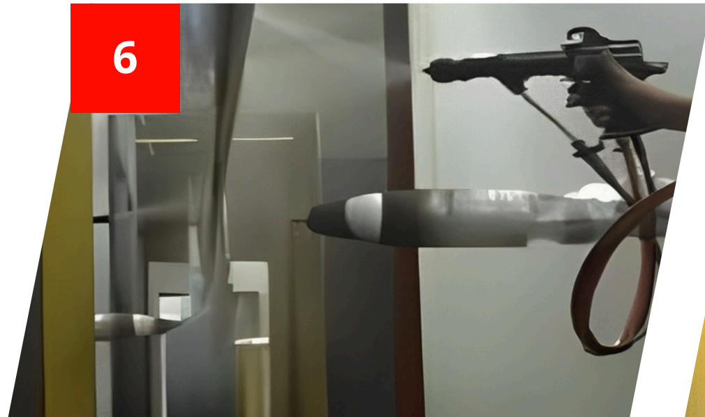
Wet Paint - Top Coat
